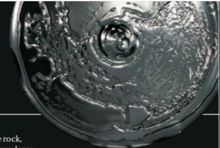
▲ This silicon boule was pulled out of the melting pot prematurely. We're seeing the underside, where molten silicon dripped off.
